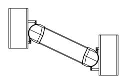
2) SLIDE THE ENTIRE RAIL ASSEMBLY BETWEEN THE POSTS AND ATTACH THE BRACKETS TO THE POSTS USING THE SUPPLIED SCREWS
